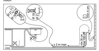
It makes no difference which way the drain hose faces, either to the right or left of the dishwasher.
